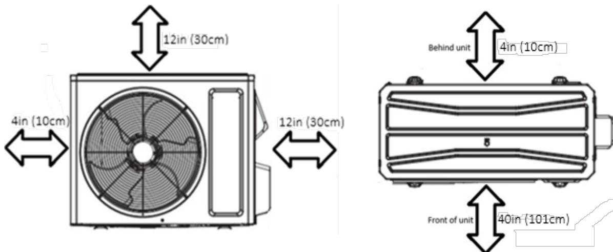
Unit must be placed a minimum 18in (45cm) above any surfaces to allow for snow clearance and defrost runoff.
