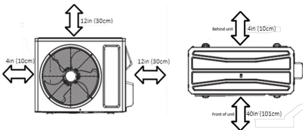
Unit must be placed a minimum 18in (45cm) above any surfaces to allow for snow clearance and defrost runoff.
