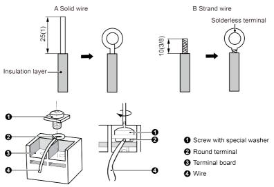
(3) How to connect the communication wires and power cords.
