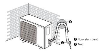
(3) In heating mode, the outdoor unit discharges condensate. Position the drain hose to prevent structural damage and sidewalk icing.
