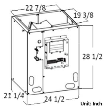
Control board can be moved according to installation needs
