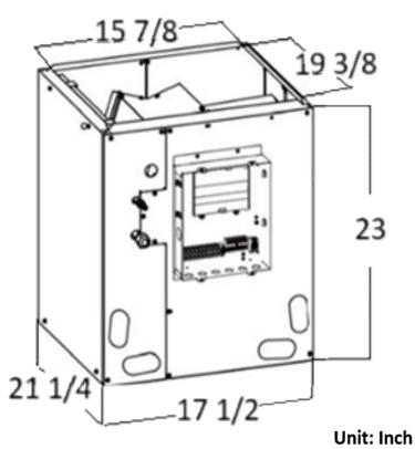
Control board can be moved according to installation needs
