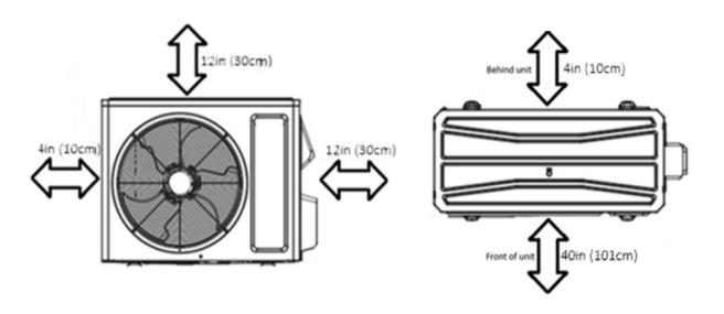
Unit must be placed a minimim 18in (45cm) above any surfaces to allow for snow clearance and defrost runoff.
