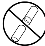
Do not crimp service valve connector when pipe is smaller than connector
