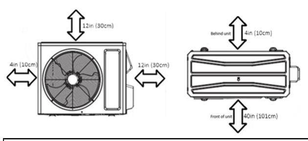
Unit must be placed a minimim 18in (45cm) above any surfaces to allow for snow clearance and defrost runoff.
