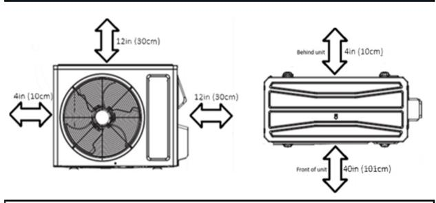
Unit must be placed a minimim 18in (45cm) above any surfaces to allow for snow clearance and defrost runoff.
